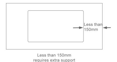
The distance between a cut-out and an edge or join must be no less than 60mm. The greater the distance, the stronger the area. For cut-outs which result in less than 60mm rails either to the front or back, important consideration should be given to making these rails from separate pieces to avoid issues with cracking. Please advise the cabinet manufacturer and/or customer that separate rails should be used and the reasoning behind it.
