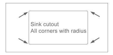
If the distance between the cut-out and a joint is less than 150mm, the area needs to be supported. This can be achieved by ensuring that all joints are placed at the junction of the base cabinets or fitting a solid support under the joint.
